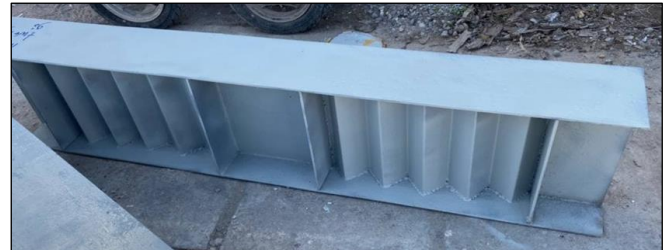
Fig. 8 Beam with corrugate web two layer and thickness 1 mm (B3).
