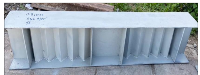
Fig. 10 beam with corrugate web two layer and thickness 0.5 mm (B5).
