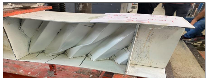
Fig. 38 Diagonal corrugated beam with thickness 1 mm (B7).
