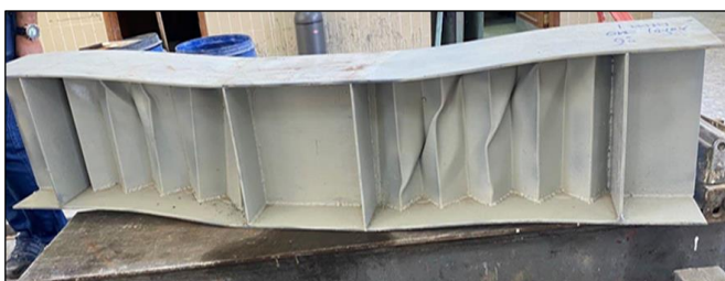
Fig. 33 Corrugated beam with one layer thickness 1 mm (B2).
