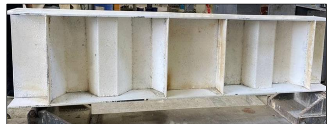
Fig. 11 Beam with trapezoidal corrugate and thickness 1 mm (B6).
