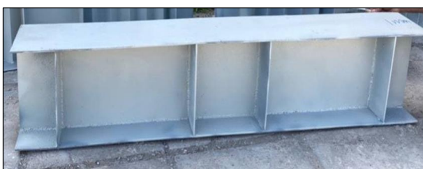
Fig. 6 Control model without corrugate web (B1).
